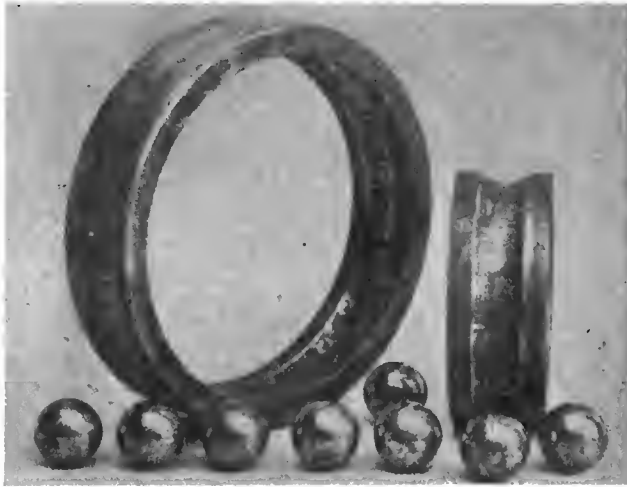
EFFECT OF ACID AND RUST ON BALLS AND RACES.
